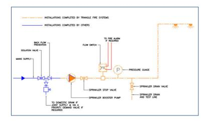
This sprinkler supply system is as per Type 1 but with the addition of a booster pump. Booster pumps can only be used when there is sufficient flow but not sufficient pressure. Additionally, permission must be gained by the water supplier. However, where the water tank is on the roof then this system can also be used and permission from the water supplier.
