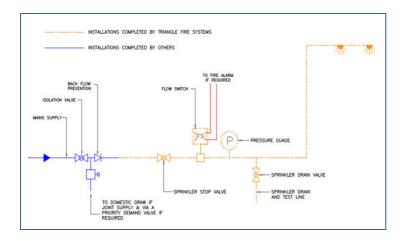
A water supply is brought into the building which may be dedicated to the sprinkler system or serve both the sprinkler system and the domestic draw. This type of supply is extremely reliable and normally cost effective.
