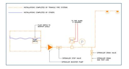
When the current water supply is insufficient and the addition of a separate water supply from the main does not have sufficient pressure/flow, then a dedicated sprinkler tank should be installed. This tank can have the addition of an infill of simply filled up with a hose and monitored via the float switch.
